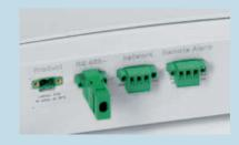
Volt-free contact and RS 485 serial interface for external temperature and alarm documentation plus interface for a NTC temperature probe.
